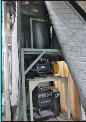
(2) 7.5-HP Conair Model CF-14 Granulators w/ Air Locks, Cyclones and Hoppers
