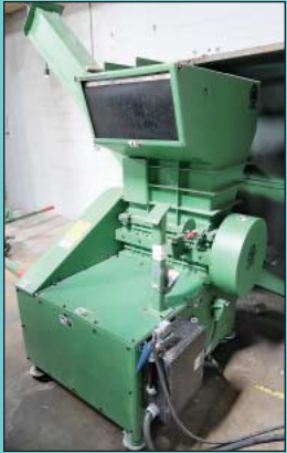
50-HP - 12" x 18" Rapid Model 600C Heavy-Duty Granulator w/ Sound Enclosure
