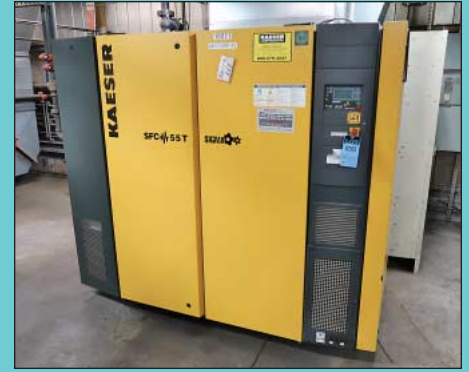
75-HP Kaeser Model SFC-55T Air Compressor w/ Built in Dryer
